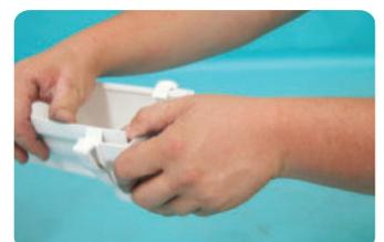
When clipping gutter corners, unions or end caps; firstly unclip then squeeze guttering into joint until fully seated on the gasket. Then reclip into place.
